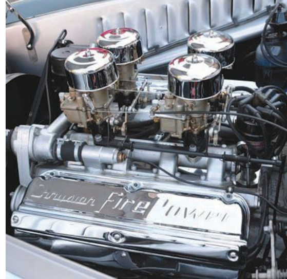
This Hemi utilizes the four-Weber intake manifold created for a later series of Cunningham "continuation" cars. Some '50s originals used a similar unit, mounting four Zenith one-barrel carburetors.
