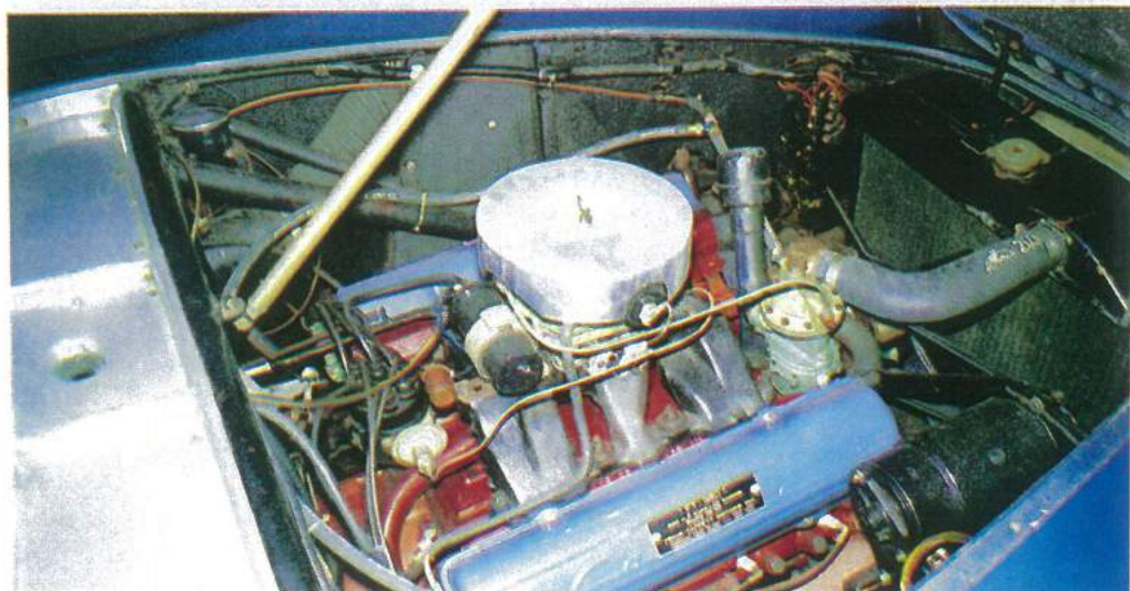
Top: The C-1's dashboard was utilitarian. Middle: Considered "lavishly appointed," the cockpit had $300 leather bucket seats. Bottom: Though the C-1 was powered by a 331-cubic-inch Cadillac engine, later models were to rely primarily on Chrysler power. Opposite page: The lines of the C-1 were the result of what its builders liked.
