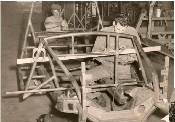
Above: The integrated roll bar on this chassis indicates that it is s/n 5206, the only coupe bodied in West Palm Beach. After the first car, all Cunninghams utilized Chrysler's 331 cu. in. Hemi with a log manifold designed and built by Cunningham. two Cadillacs, one a slightly modified Coupe de Ville
