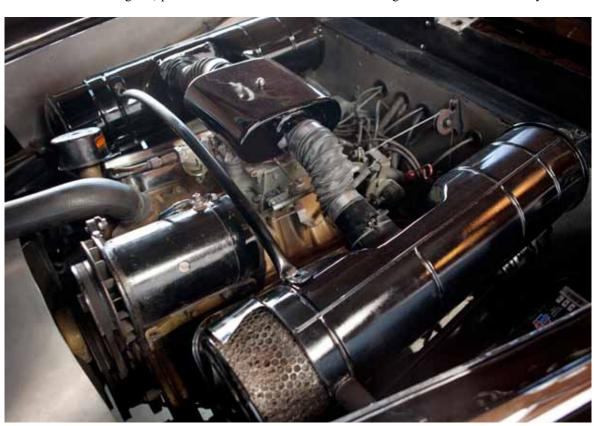
Above and right: The only Cunningham C-3 that has remained in family ownership is this black coupe, built originally as the factory demonstrator. This is also the only car equipped with a single 4 bbl. carburetor and special air cleaners, instead of the Cunningham log manifold and four carburetors.
