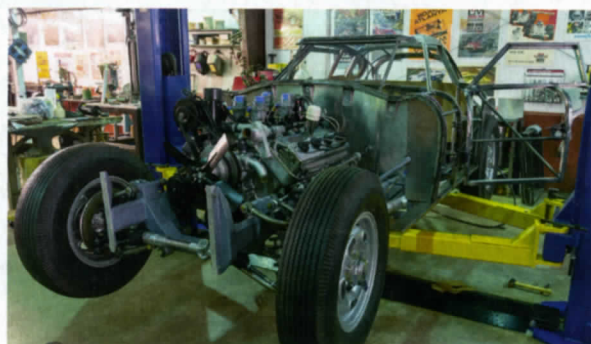
This page Aluminium panels are spot-on thanks to the digital scans taken from the original car, and engine is a correct '52 Hemi complete with Cunningham parts.
