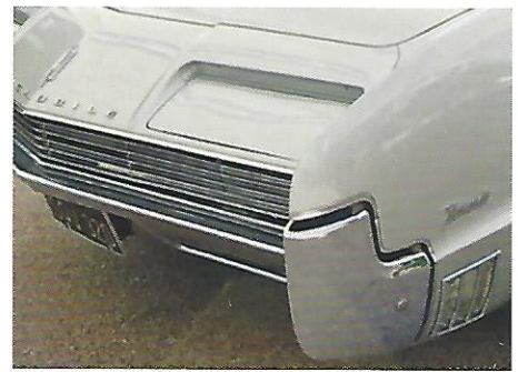
The 1966 Oldsmobile Toronado Fitch Phantom on display looked to have a 1967 headlight surrounding panel. Above is the 1966 trim with its parallel grille and the "brows" at the top of the retractable lights. The change for 1967 (top) featured a squared grille pattern and the "brows" were deleted. The Sept. 1966 issue of Popular Mechanics featured a two-page article on the Fitch Phantom where the headlight "brows" are clearly visible on the picture of the car in the article.
