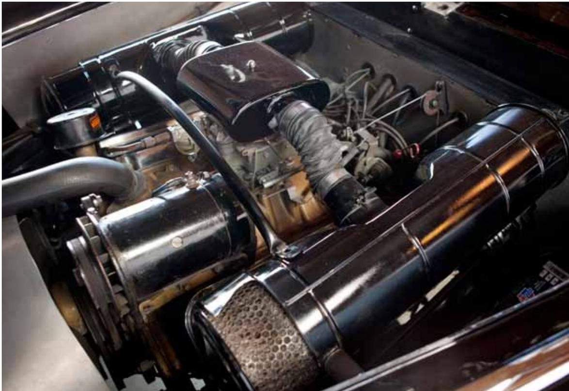
Above and right: The only Cunningham C-3 that has remained in family ownership is this black coupe, built originally as the factory demonstrator. This is also the only car equipped with a single 4 bbl. carburetor and special air cleaners, instead of the Cunningham log manifold and four carburetors.
